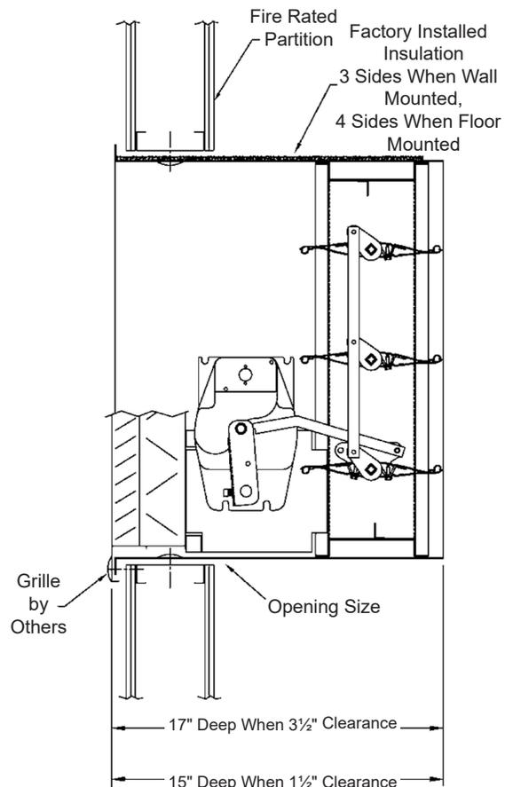
Combination Fire/Smoke Damper • 1½ Hr. Rated • Airfoil Blade • Leakage Class II • 250°F or 350°F Rated • Front Grille Access • Galvanized Steel
