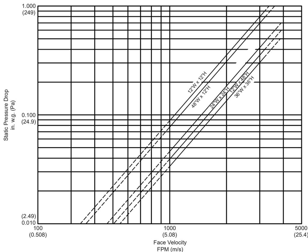
Sizes listed on this chart exceed the size limitations of the UA2GF. These sizes are based on the model UA2 approval.
